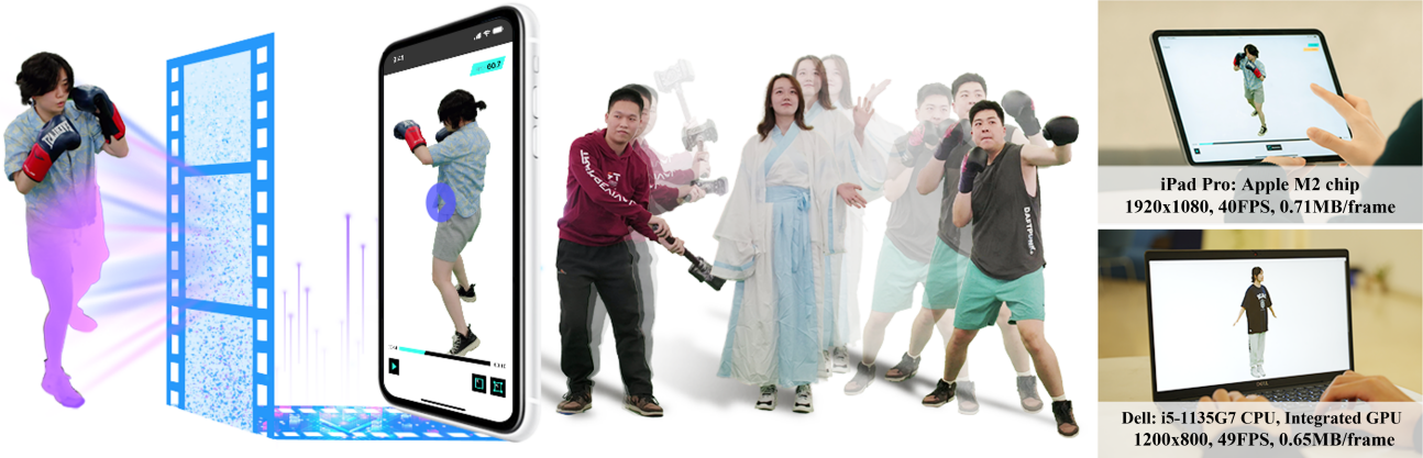
Figure 1. Our proposed VideoRF views dynamic radiance field as 2D feature video streams combined with deferred rendering. This technique facilitates hardware video codec and shader-based rendering, enabling smooth high-quality rendering across diverse devices.
